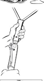
1. Install Big Shot head into the (female) end of a Jameson fiberglass extension pole. Secure by aligning the two holes and fully engaging the spring loaded pin.
