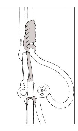
Karabiners incorporating a pulley e.g. DMM Revolver increase the efficiency of the system when used to hang the load. It's never been so easy (for the climber) to get
