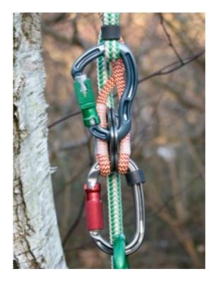
attachment. An Oval here has the advantage that it can accept wider loads at both ends, so it can be rotated if desired. And the load from the splice is transferred through the rigging plate of the pulley to a central position on the Oval karabiner where the loading pattern is now 1/4-1/2-1/4, which plays to its strengths. Oval karabiners loaded like this often break at well above their rated MBS
