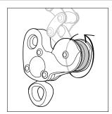
• Check the condition of the swivel (cracks, deformation...).
