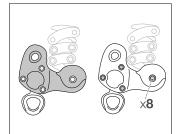
• Check for wear at the points where the friction chain stops against the frame. Look for sharp edges that could damage your rope. If necessary, round any sharp edges with fine-grain sandpaper.
